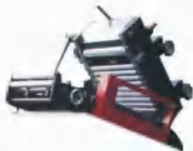
上滚轮座可作掀开式 方便清理滚筒 The upper roller seat can be opened Easy to clean the drum
