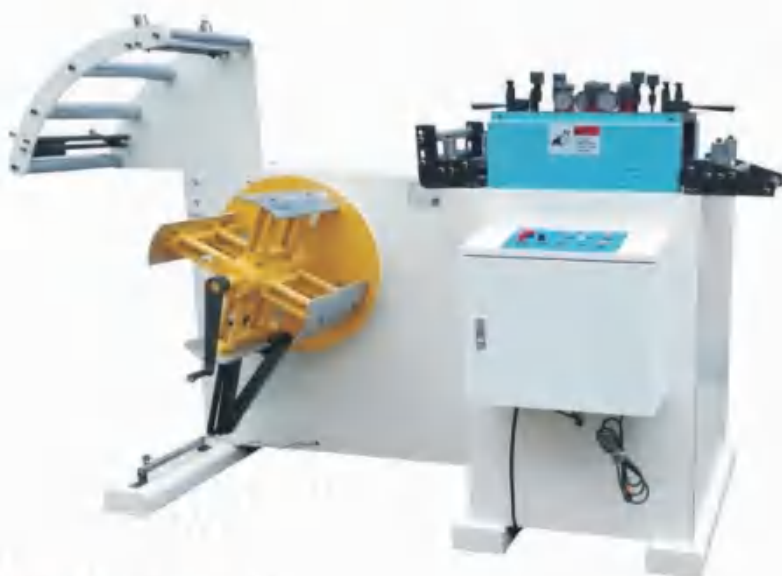
上滚轮座可作掀开式 方便清理滚筒 The upper roller seat can be opened Easy to clean the drum
